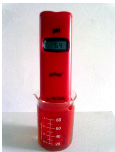
Image 5.0: Measurement of pH of 1% w/v aqueous solution of powdered bark by pH meter (Standard glass electrode, pHep-HI98107, Hanna Instruments, Mauritius)
