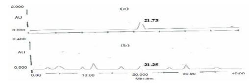
Figure 5. HPLC Chromatogram of (a) eugenol and (b) *Ocimum sanctum*. Mobile phase was 80% Diluted water (with 1% acetic acid) and 20% Acetonitrile at pH 6.5; analytical column: Inertsil 7 ODS-3 4.6 mm i.d. x 250 mm; 1 ml/min; 25°C; injection volume: 5µL; detection at 280 nm.
