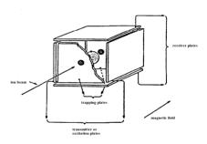
Figure 2: FTICR- Mass Spectrometer
