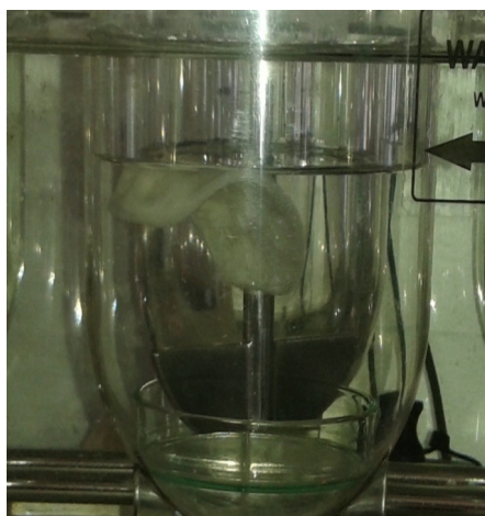
Figure 10: Gel Formation from sodium alginate based IGSs F4 in dissolution apparatus
