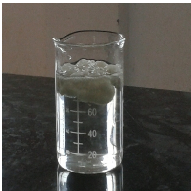
Figure 8: Gel Formation from sodium alginate based In situ solution F4 of MLX in pH 1.2 buffer
