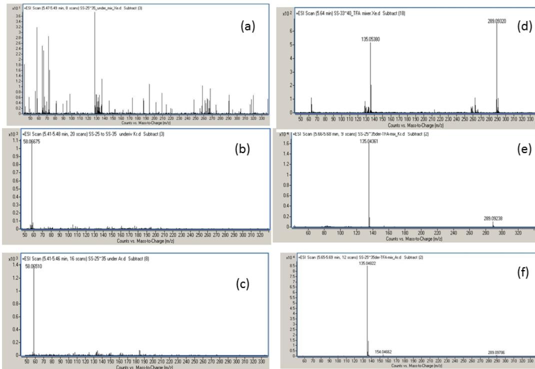
Figure 3. Xe-, Kr- and Ar-MPPI mass spectra of the underivatized and the TFA-derivatized methedrone. (a) Xe/underivatized, (b) Kr/underivatized, (c) Ar/underivatized, (d) Xe/TFA-derivatized, (e) Kr/TFA-derivatized, (f) Ar/TFA-derivatized.
