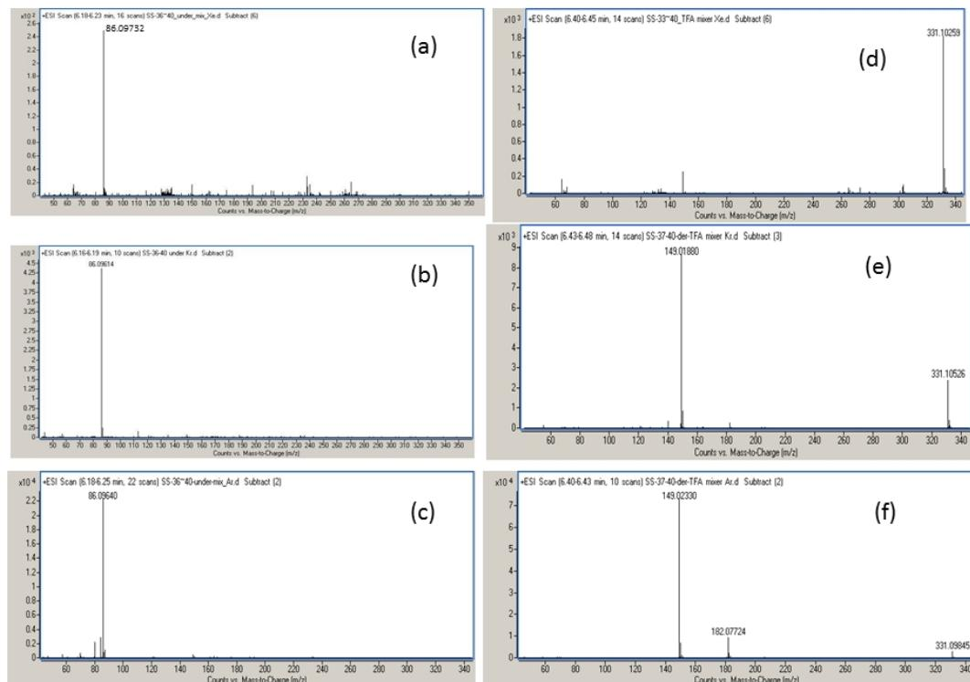
Figure 7. Xe-, Kr- and Ar-MPPI mass spectra of the underderivatized and the TFA-derivatized pentylone. (a) Xe/underderivatized, (b) Kr/underderivatized, (c) Ar/underderivatized, (d) Xe/TFA-derivatized, (e) Kr/TFA-derivatized, (f) Ar/TFA-derivatized.
