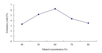
Figure 1: Effect of the ethanol concentration on the extraction yield of flavonoids
