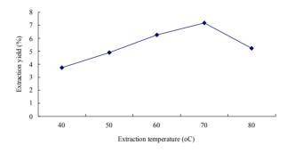
Figure 4: Effect of the extraction temperature on the extraction yield of flavonoids
