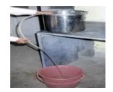
Decantation process (Water is being removed using siphon)
